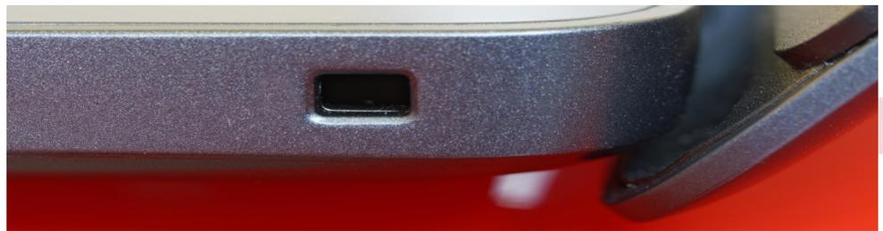
Typically on the side or front base of the laptop, this little port is called a Kensington Security Slot. It's designed to work with a Kensington Lock/Cable to physically secure the device to an anchor point.
