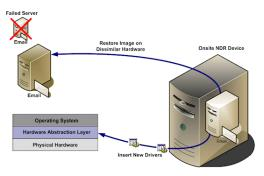
device can perform a Bare Metal Restore. The Virtual Server will be loaded onto the physical hardware, regardless of hardware changes. New drivers will be inserted automatically if necessary.
