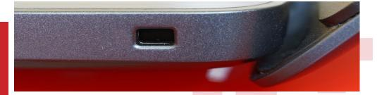
Typically on the side or front base of the laptop, this little port is called a Kensington Security Slot. It's designed to work with a Kensington Lock/Cable to physically secure the device to an anchor point.
